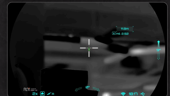
▲ ① Function ON → ② LRF Rangefinding → ③ Ballistic Solution
